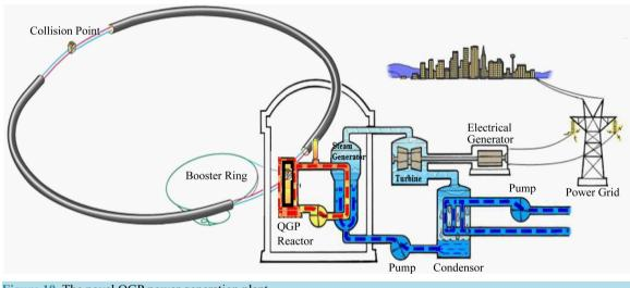
Figure 10. The novel QGP power generation plant.
