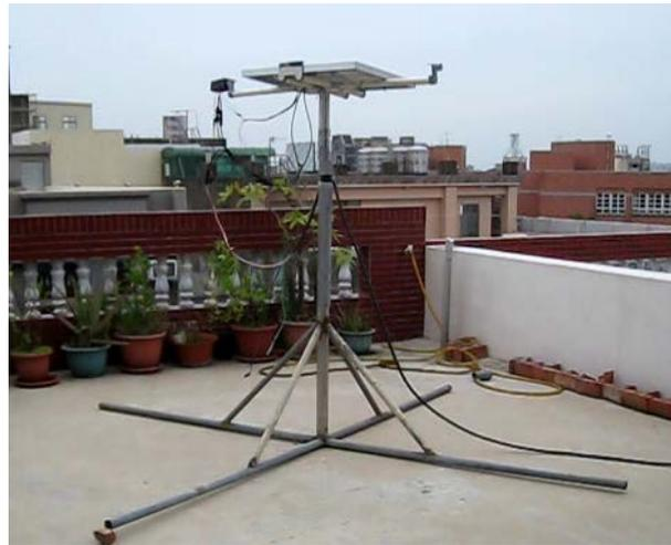
Figure 6. The tracking device for a solar cell.
