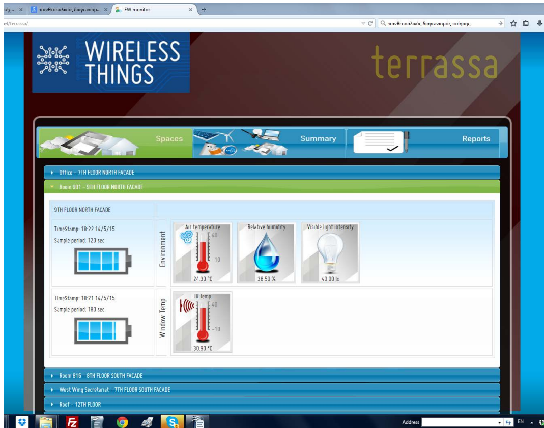
Figure 4. The monitor dashboard for the Terrassa hospital ( http://wsn.energywarden.net/terrassa ) where the inner ambient temperature as well as inner, IR scanned, wall temperature values are reported. In another screen the outdoor temperatures and the wind speed are shown.
