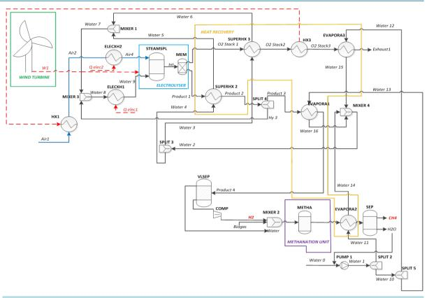
Figure 2. Flow diagram of the wind turbine coupled with HTSE and combined with methanation unit.
