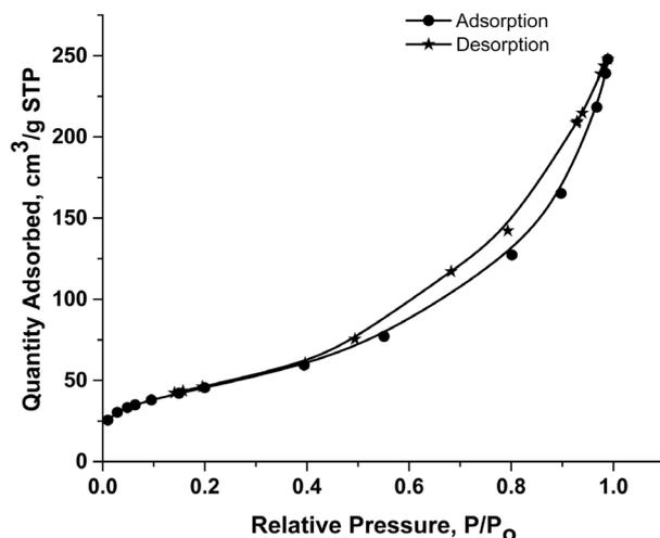
**Figure 1.** Nitrogen adsorption/desorption isotherms of Z-TiO<sub>2</sub> at -196°C.
