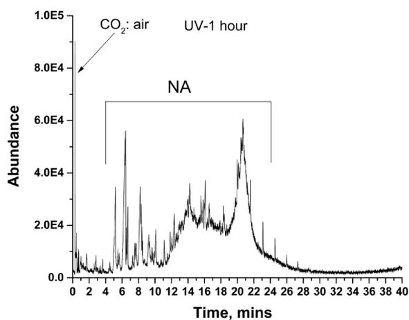
**Figure 6.** GC spectra of headspace gas from UV irradiation on Z-TiO<sub>2</sub> and naphthenic acid at 25°C for 1 hour.
