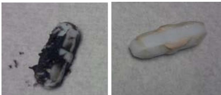
**Figure 9.** Appearance of stir bars from a mixture of Z-TiO<sub>2</sub> and naphthenic acid (Right) after exposure to UV light for 5 days and (Left) kept in dark for a week.
