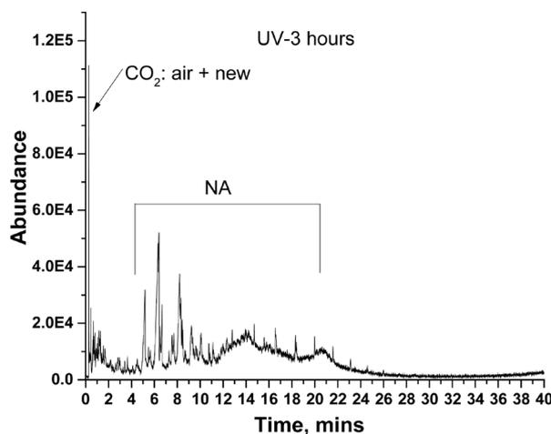
**Figure 7.** GC spectra of headspace gas from UV irradiation on Z-TiO<sub>2</sub> and naphthenic acid at 25°C for 3 hours. Abundance of CO<sub>2</sub> has increased compared to dark conditions.
