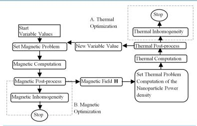
Figure 2. Flow chart for thermal and magnetic coupled uniformity search.
