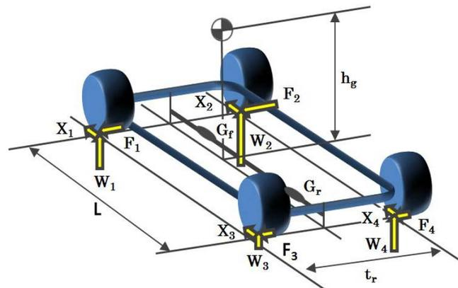
**Figure 3.** Model for the analysis of load distribution [11].
