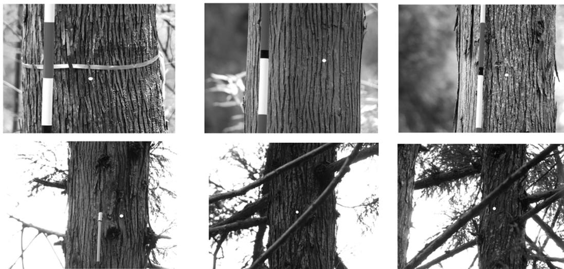
**Figure 3.** Measuring stem photographs of No. 5 in Plot 3 (white dots indicate red dots of laser pointer).
