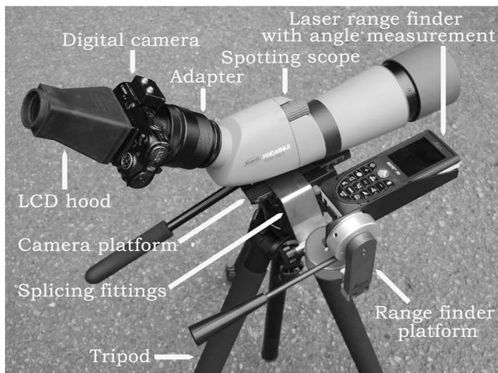
**Figure 1.** Digital-scope photography system (DSPS).
