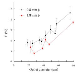
Figure 5. Comparison of transmittance through the capillary between the 1.8 mm and 0.8 mm inlet diameters at 633 nm.
