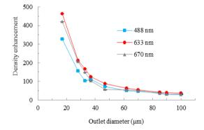
Figure 7. Density enhancement of the capillary for the 1.8 mm inlet diameter as a function of the outlet diameter without the optical lens.
