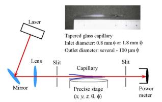
Figure 1. Experimental setup for transmittance measurements.
