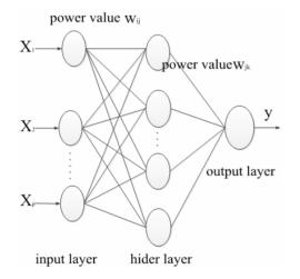
Figure 1. Schematic diagram of BP neural network.
