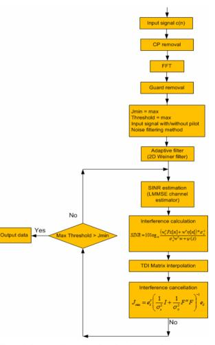
Figure 4. Proposed combination signal processing technique of ICS for 3GPP/LTE.
