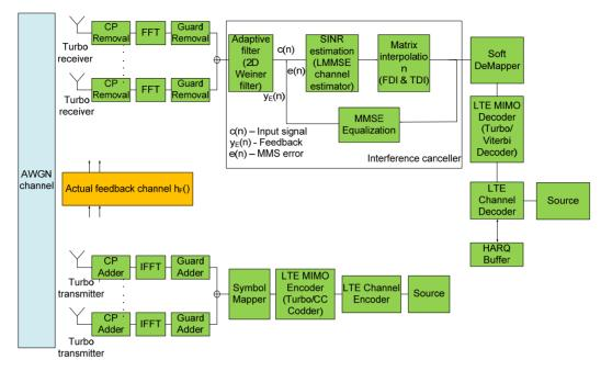
Figure 3. Proposed system model of ICS Repeater without Pilot signal for 3GPP/LTE.
