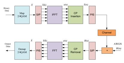
Figure 1. The block diagram of an OFDM system.
