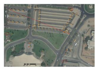
Figure 5. Location of maximum errors due to affine transformation tool.
