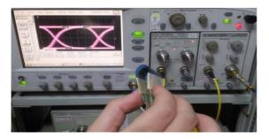
Figure 11. 2.5 Gb/s eye-diagram per channel for the FOW typed EPCB at  $180^{\circ}$  bend.
