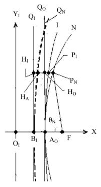
Figure 2. Paths of the corpuscle.  $Q_o$ : tangent line,  $Q_N$ : directrix in the curved space,  $Q_I$ : original directrix.
