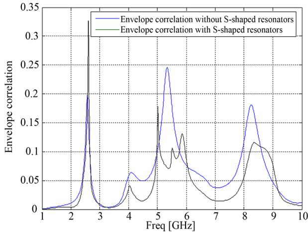
Figure 7. Simulated correlation with and without S-shaped resonators.
