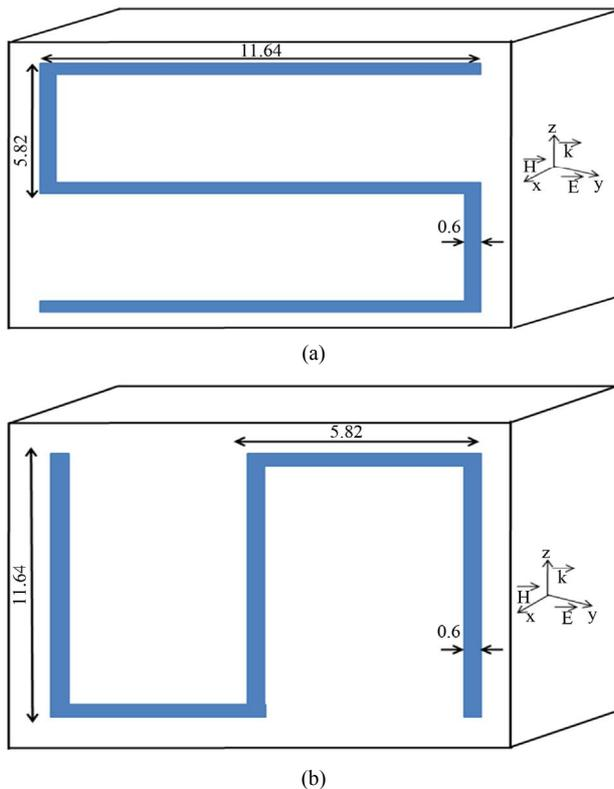
**Figure 3. Design of the two forms of the proposed S-shaped resonator. (a) First form; (b) Second form.**
