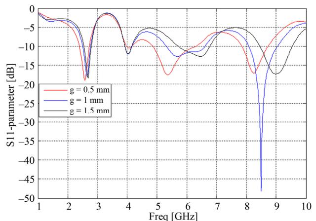
Figure 2. The effect on operating frequency due to the use of the gap.
