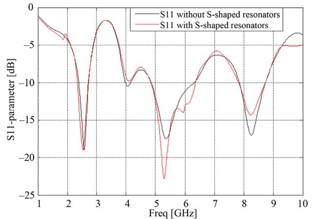
Figure 6. Simulated return loss with and without S-shaped resonators.
