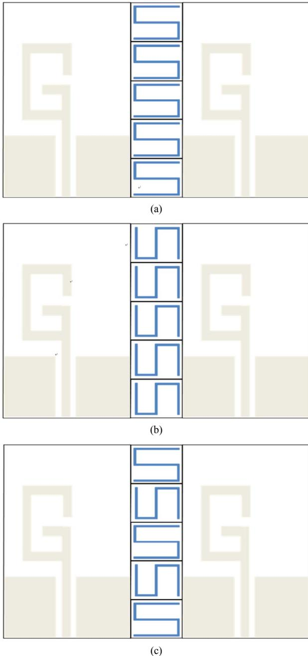
Figure 4. Different configurations of array antenna using S-shaped resonators. (a) Case 1; (b) Case 2; (c) Case 3.
