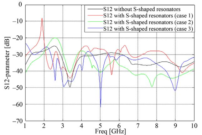
Figure 5. Mutual coupling with and without S-shaped resonators.
