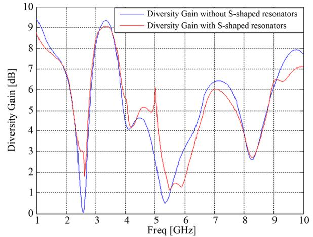
Figure 8. Simulated diversity gain with and without S-shaped resonators.
