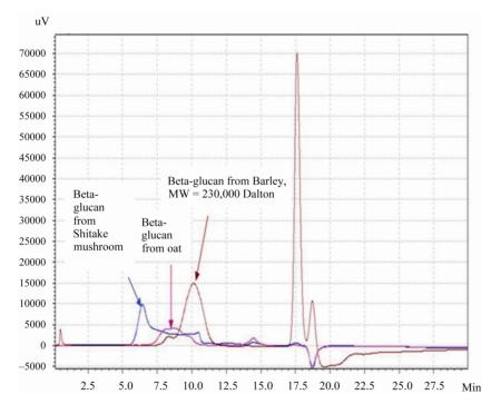
Figure 4. The high performance liquid chromatography (HPLC) profiles of  $\beta$ -glucan solutions extracted from oat and shitake mushroom and pure  $\beta$  D-glucan from Barley.
