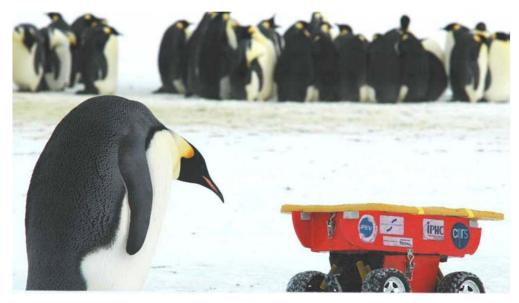
**Figure 4.** UGV deployed at Dumont D'Urville, Adélie Land, Antartica to perform observations of breeding Emperor penguins (*Aptenodytes forsteri*). Courtesy Yvon Le Maho.
