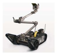
**Figure 1.** Morphology of an UGV (iRobot<sup>®</sup> 510 PackBot<sup>®</sup>). This small ROV ( $88.9 \times 52.1 \times 17.8$  cm; 10.89 kg without batteries) can be used on a great variety of terrain (image courtesy iRobot<sup>®</sup>).
