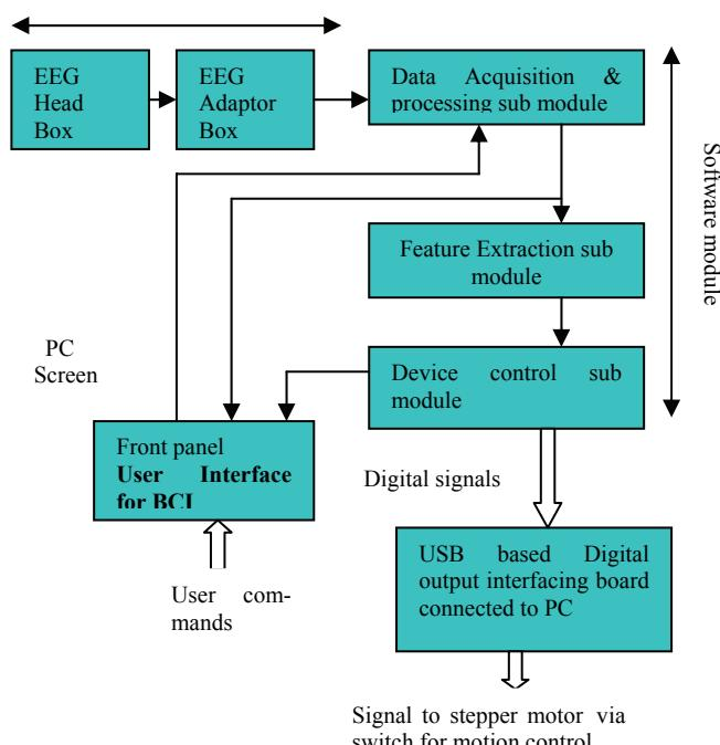
**Figure 3.** Functional elements of a BCI system EEG hardware interfaced to PC
